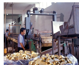
metal plating operation
